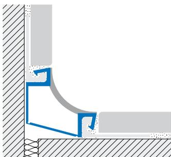
**COFLEX CR** is expressly conceived to perimeter joint wall/floor coverings supplying sufficient elasticity for the expansion and meeting the cove base hygienic corner cleanliness requirements. It also serves as a sound breaker of the covered surfaces so that trampling of foot steps is not transmitted to the adjacent walls.
